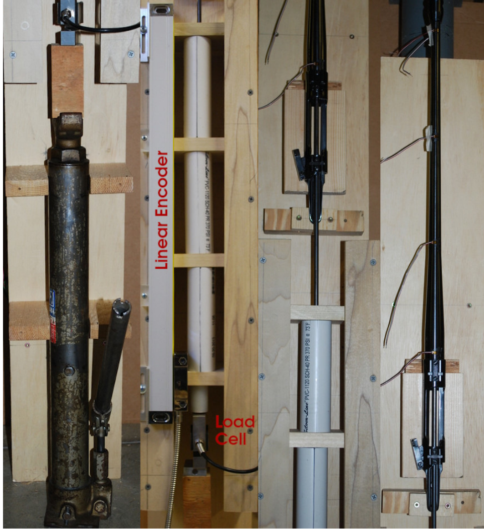
Figure 13: Bullet pusher test fixture illustrated in four sections.
