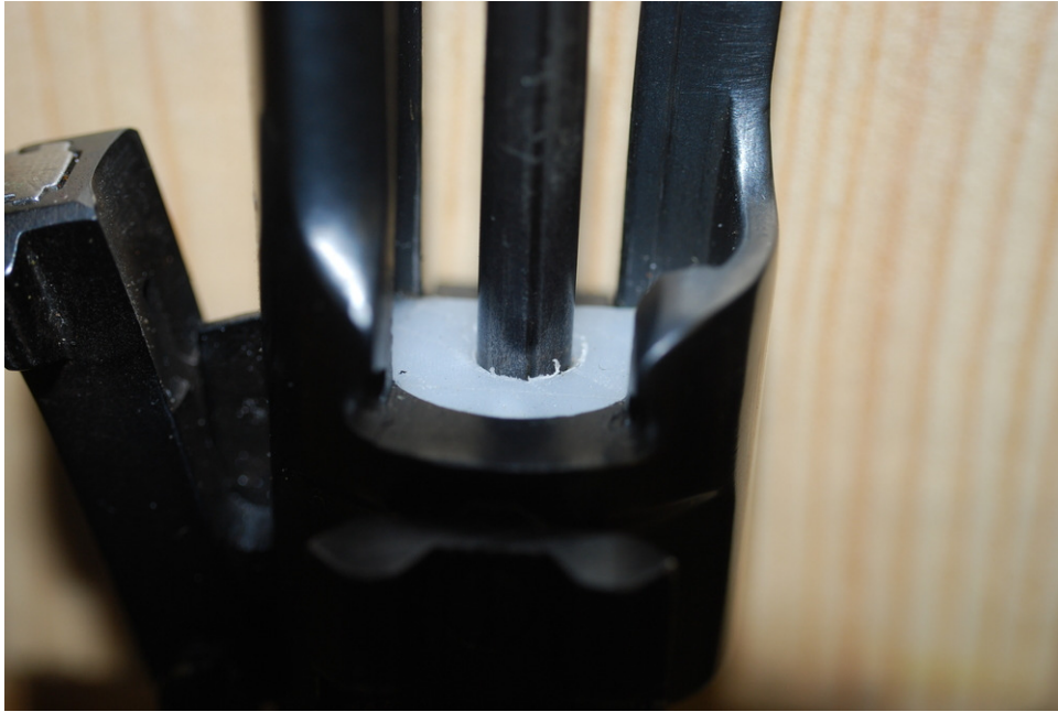
Figure 15: Illustration of nylon bushing to assist in keeping coaxial alignment of the pushing rod.
