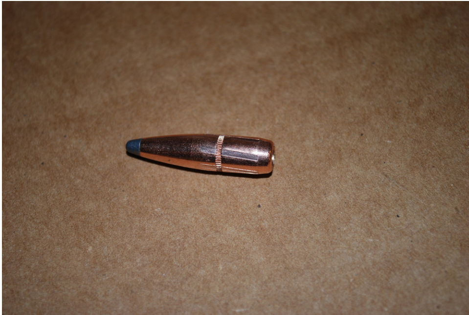
Figure 19: Illustration of engraved bullet after being pushed through the whole bore length.
